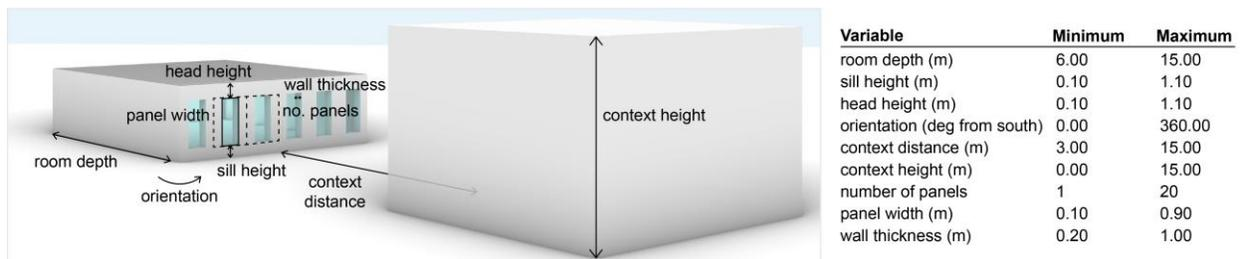
Figure 3: Common design space: daylight room on building facade
