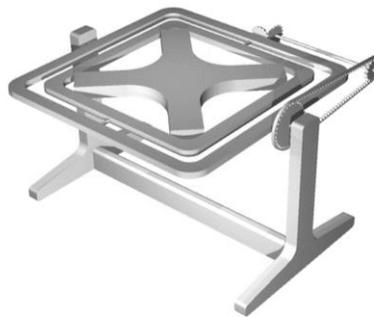
Figure 2: A biaxial rotational machine with an X-shaped mold at the center.
