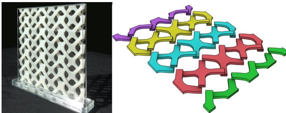
Figure 6: Intertwined photobioreactors as a building façade (left) and the Modular break-up of the facade to fit the size of a rotational molding machine (right).
