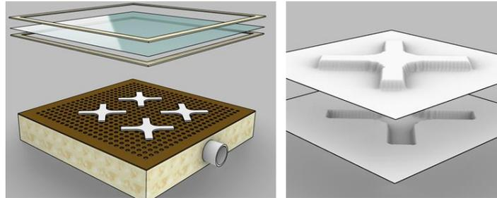
Figure 1: Fabrication methods, e.g. vacuum forming (left), that create two halves (right) and the seam needs to be sealed afterward.
