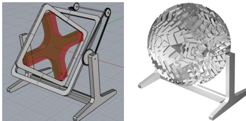
Figure 4: Discretization of the interior surfaces of the mold (left) and the cumulative rotation of the X-shaped mold (right). The two rectangular frames on the right image are hidden.
