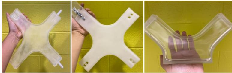
Figure 11: Cast models with three different types of resin: Smooth Cast 325 (left), Innothane IE-3025 (middle), and Crystal Clear 202 (right)
