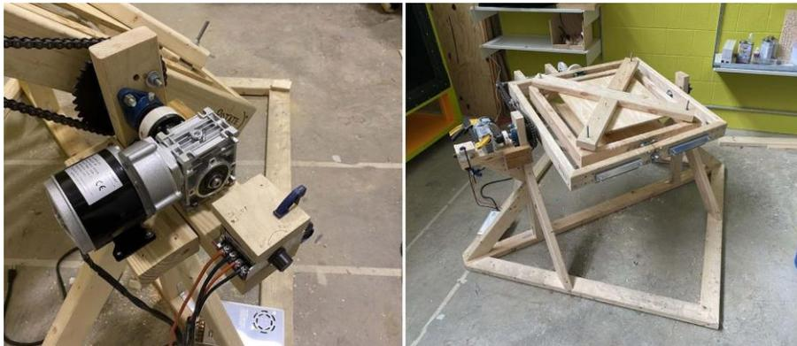
Figure 8: Highlighted modifications and improvements of rotational molding machine.
