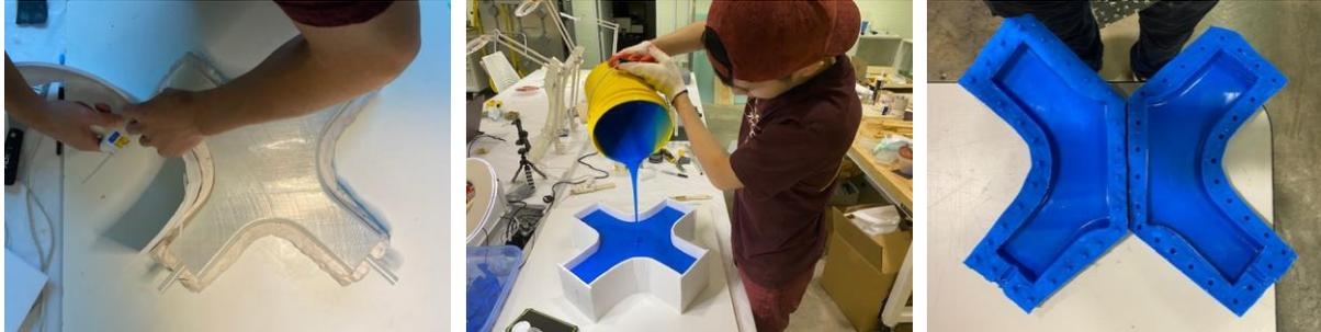
Figure 9: Mold making process. Claying the 3D printed object (left), casting one side of the mold with Mold Max 30 ( middle), and the cast two halves of the rubber mold (right).
