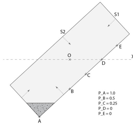
Figure 3: A hypothetical scenario that liquid material coats a rectangular geometry using a rotational molding machine.
