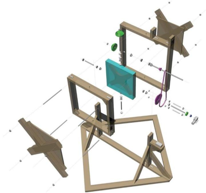
Figure 7: Digital fabrication model of the rotational casting machine.
