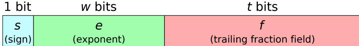
Figure 1: General floating-point binary encoding.
