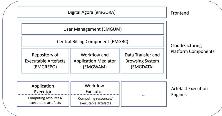
Figure 5: High-level architecture of the CloudiFacturing Solution.
