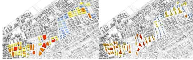
Figure 1: Left: Heat map of Low-Performance EPN with demand; Right: Heat map of High-Performance EPN with demand; red in the heat map indicates high energy demand while blue denotes low energy demand
