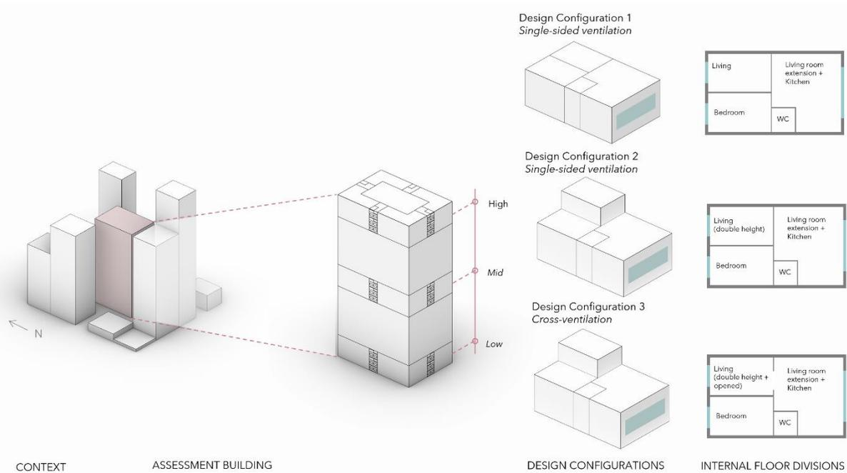
Figure 1: Apartment Set-up Design Configurations
