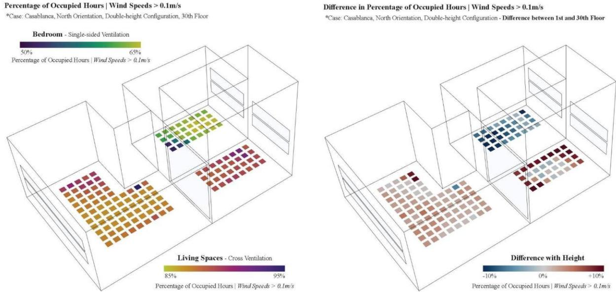
Figure 4: Deviation between simulated internal wind speeds and constant assumption of 0.1m/s
