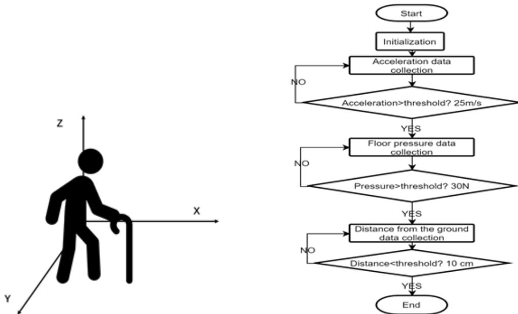
Figure 2: SEMS Fall detections: a) 3D axis movement of the person; b) the Fall Detection Algorithm using flowchart.
