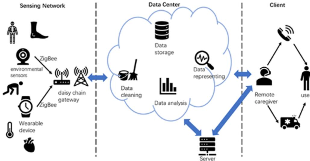
Figure 3: Overview of SEMS with 3 main components: Sensing, Computing, Monitoring.
