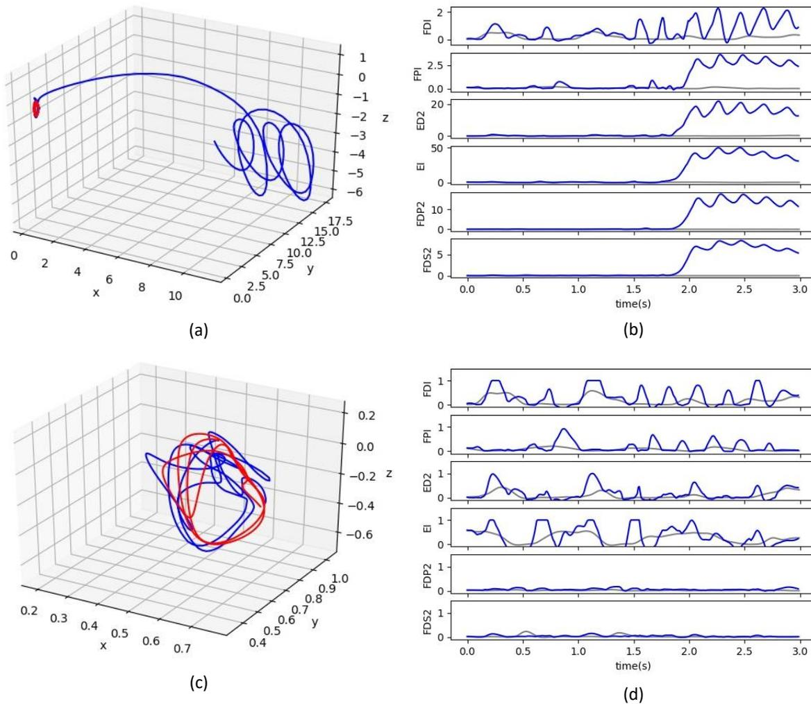
Figure 7. Top two plots show an example of an unstable scenario where (a) trajectories (red for desired and blue for simulated without error compensation) and (b) the predicted EMG (blue) and actual EMG (gray). Bottom two plots show an example of stable scenario after limiting maximum values of EMG where (c) trajectories (red for desired and blue for simulated without error compensation) and (d) the corresponding predicted EMG.
