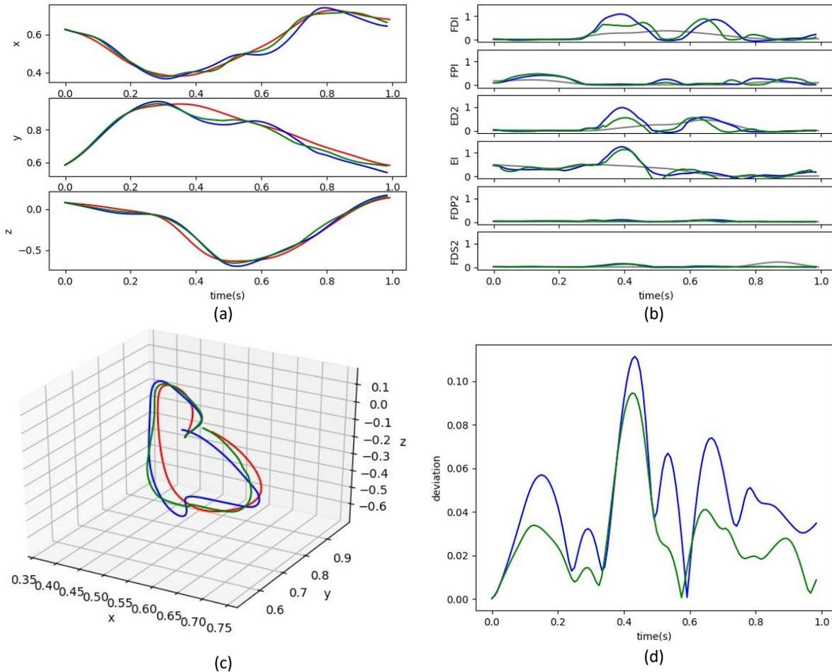
Figure 6. (a) simulated xyz positions given a desired xyz positions, (b) predicted EMG and actual (gray) EMG, (c) the corresponding 3D trajectories, and (d) deviations from the desired trajectory (where blue for simulated outcomes without error compensation, green for simulated outcomes with error compensation, and red for desired in (a)-(d)).
