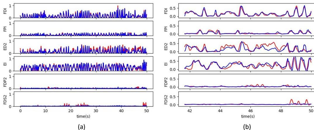
Figure 5. actual (red) and predicted (blue) EMG signals given (a) 6,000 test samples and (b) last 1,000 samples, respectively.
