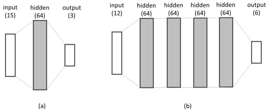
Figure 3. Fully connected ANN architectures for (a) the nonlinear system model to predict fingertip position and (b) the EMG generator.
