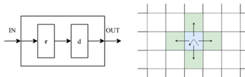
Figure 1. Cell-DEVS model. (left) atomic cell schematics; (right) 2-dimensional Cell-DEVS neighborhood.
