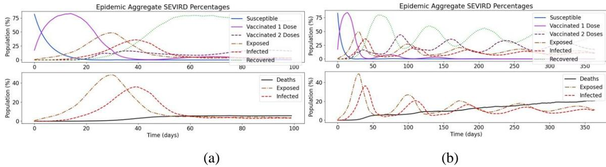
Figure. 4. Aggregate SEVIRD with vaccination enabled and no travel restriction. (a) no re-susceptibility; (b) re-susceptible.
