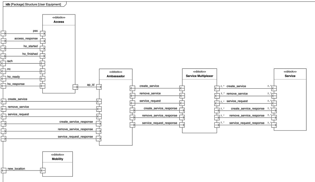
Figure 4: User Equipment Internal Block Description Diagram.
