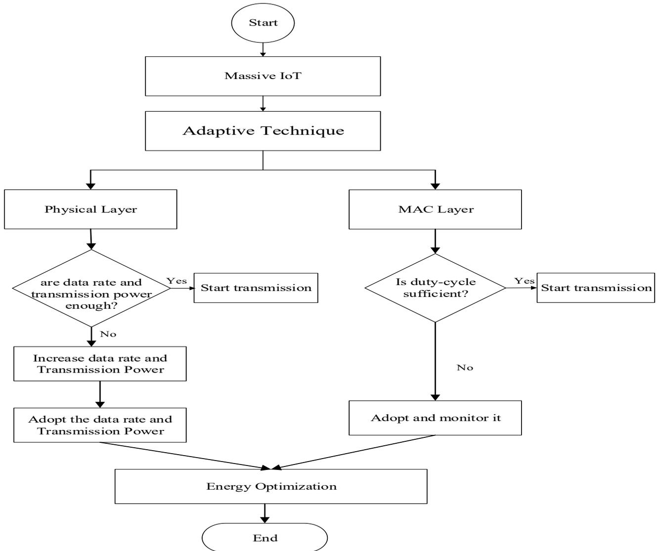
Fig. 2. Flowchart of proposed cross-layer based energy optimization algorithm in AI-based massive IoT
