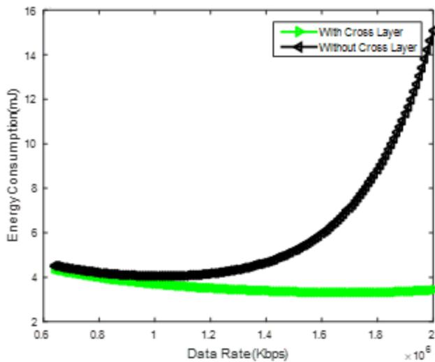
Fig. 4. Data rate vs. energy dissipation in mIoT
