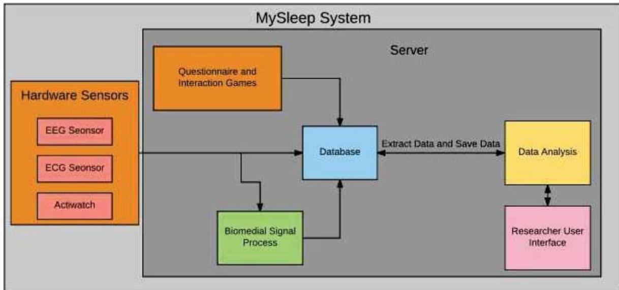
Figure 4: MySleep as a Prognosis Health Information System that can take in data from wearable sensors to measure activities, ECG waveform, and EEG waveform to further understand sleep quality.
