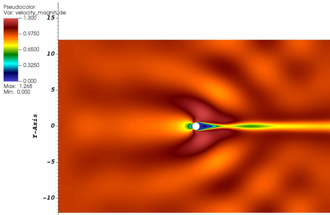
Figure 2: 2D instantaneous velocity field of flow past a cylinder at Reynolds number 180, and Froude number of 1.
