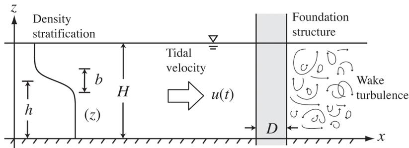
Figure 1: Schematic representation of stratified flow past a monopile. Vortices generated in the wake of the flow results in turbulent mixing (figure taken from [2]).
