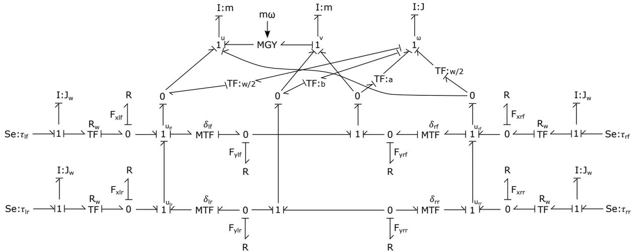
Figure 11: Bond Graph of Extended Bicycle Model
