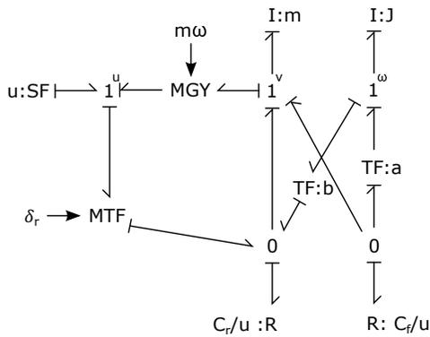
Figure 5: Bond Graph of Bicycle Model with Rear Wheel Steer
