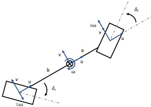
Figure 4: Bicycle Model with Rear Wheel Steer
