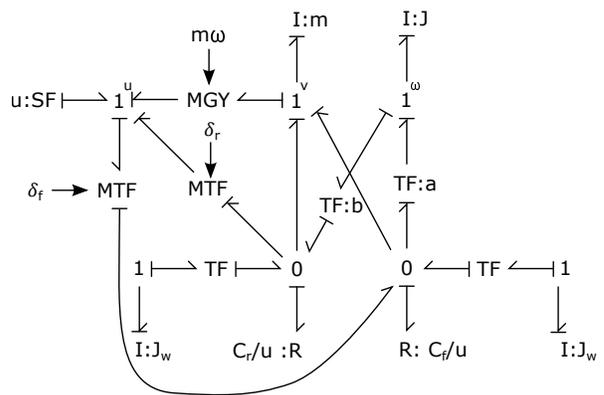
Figure 7: Bond Graph of Bicycle Model with Caster
