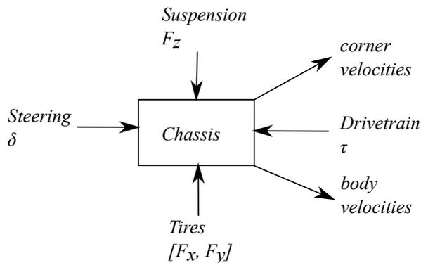
Figure 1: Vehicle Chassis Body Input/Output Relationships
