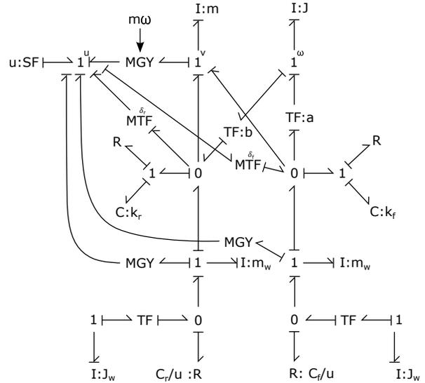
Figure 9: Bond Graph of Bicycle Model with Caster and Bushing
