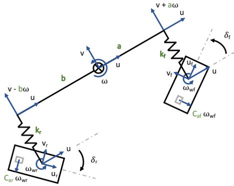
Figure 8: Bicycle Model with Caster and Bushing
