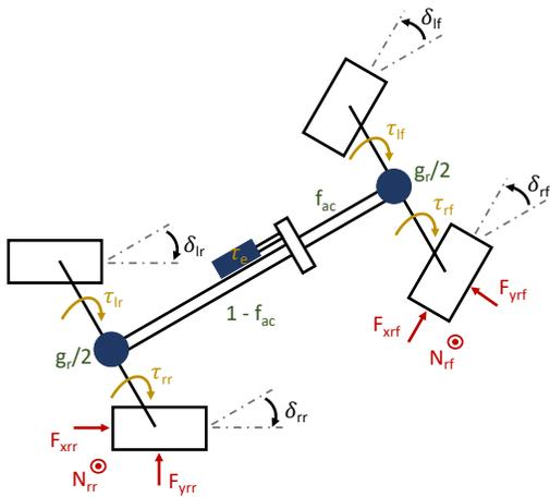
Figure 12: Extended Bicycle Model with Drive-train
