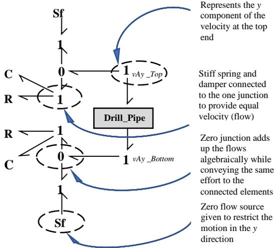
Figure 7: Boundary conditions of the BG model
