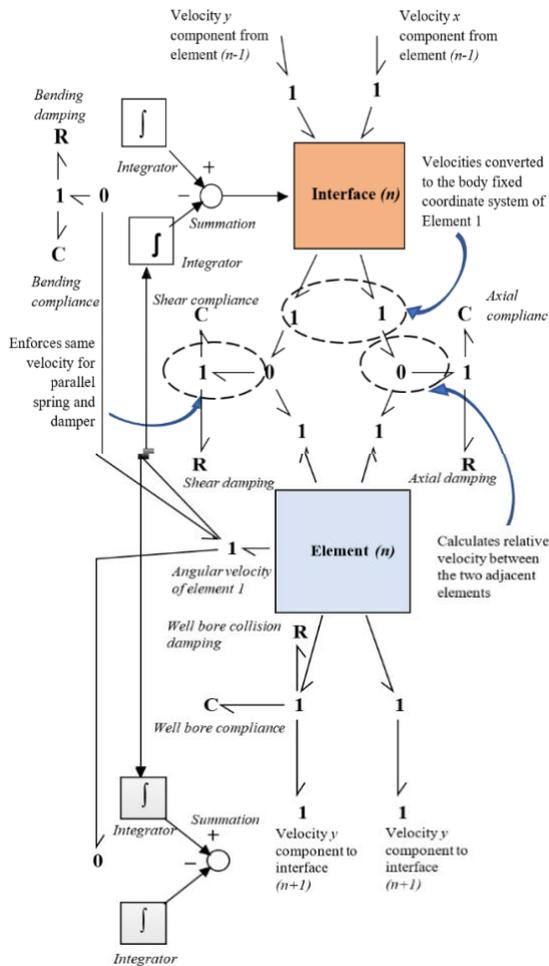
Figure 8: Repeating unit of the BG model
