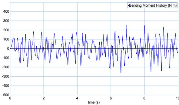
Figure 11: Bending moment fluctuation history determined through BG model
