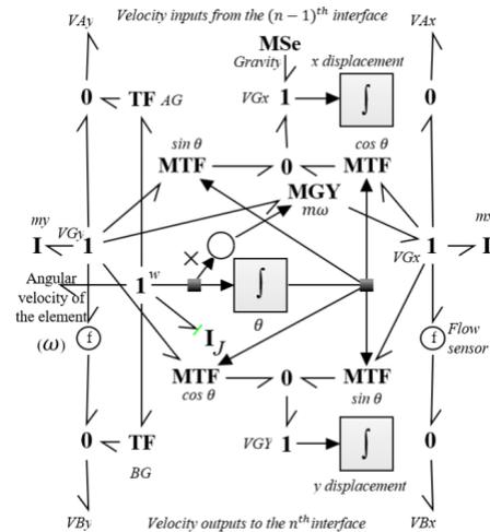
Figure 10: BG model of the 2D element
