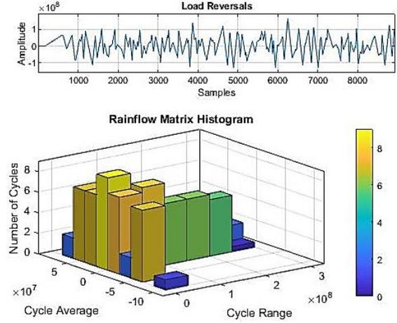
Figure 12: Rain flow counting result for a sample time of 10 s
