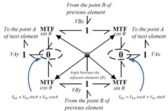
Figure 9: BG model of the Interface
