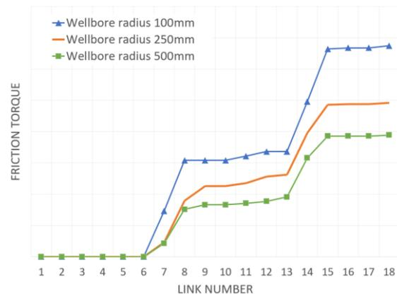
Figure 8: Frictional torque variation with changing wellbore hole radius
