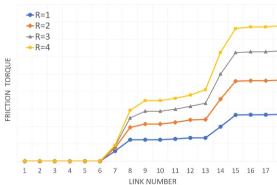
Figure 7: Frictional torque variation with changing wellbore curvature radius.
