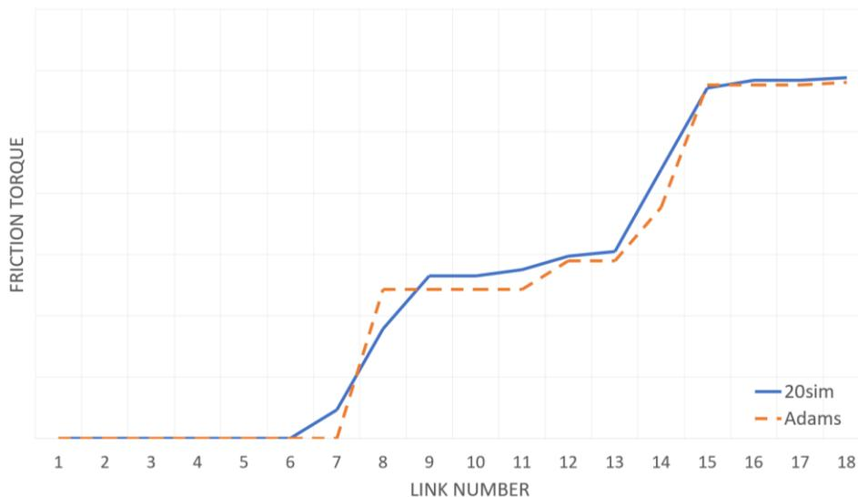
Figure 5: Comparison between the 20sim vs. the MSC Adams results for friction torque
