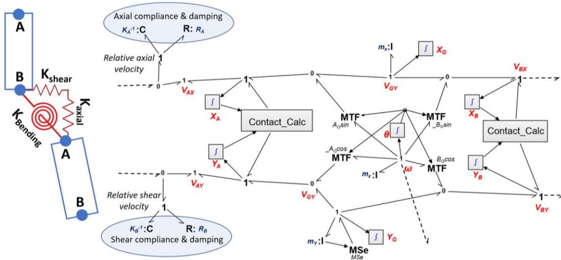
Figure 2: 20sim model of the drill string segment.
