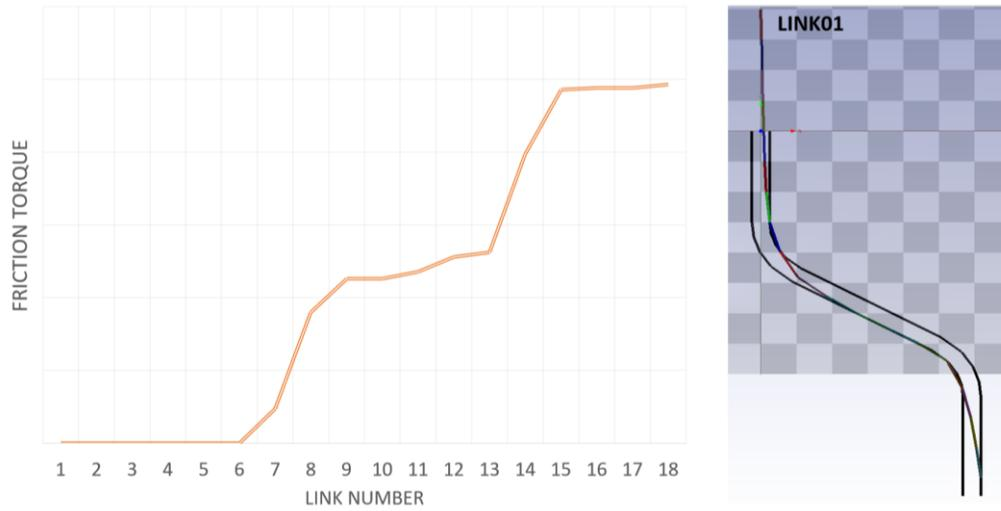
Figure 6: Torque and drag measurements from the 20sim model and output for the animation tool
