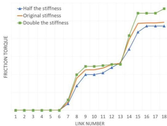
Figure 9: Frictional torque variation with changing drill string stiffness
