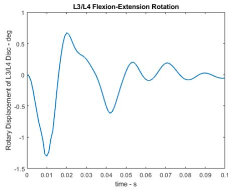
Figure 12. L3/L4 segment's rotary displacement
