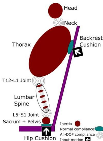
Figure 2. Schematic of the seated passenger model
